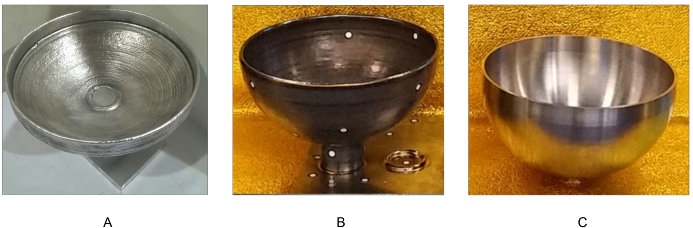
Figure 3: Case study showing three stages in creating a simple structure manufactured by WAAM; A) after WAAM operation, B) scanning and computer modelling , C) the finished item after machining.
