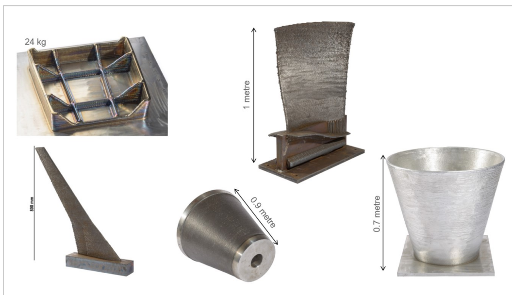
Figure 5: Semi-finished parts manufactured by WAAM
